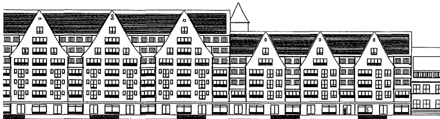
3 Conversion of a former warehouse into a residential and office building. New façade design
