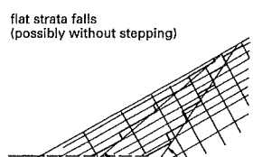
11 Rock slopes determined by the geology and jointing
