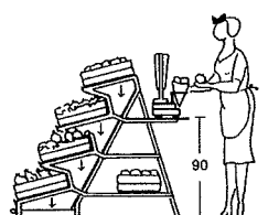
8 Counter with mounting for boxes and wire baskets; draining shelf and dirt drawer
